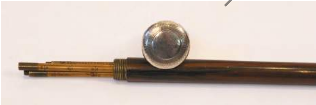
Surveyor's walking cane, with a silver knob and a three-part boxwood rule hidden in the rosewood shaft c.1923
