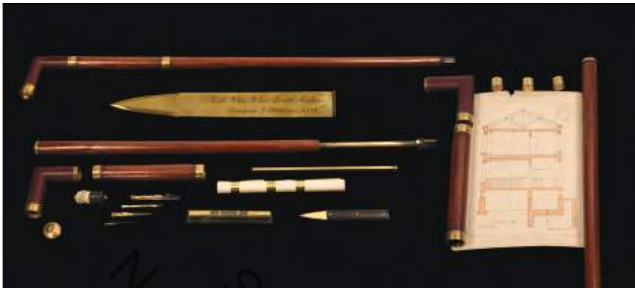
Leather clad-handled architect's cane housing a compass, a pencil and assorted drafting tools Mounted on a mahogany shaft which contains a level, a straight edge, a letter opener, a pendulum bob and architectural plans Sweden, 1892
